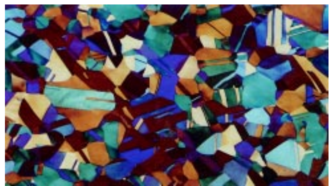
Fig 4. - Annealed and cold drawn arsenical, phosphorus-deoxidized copper prepared with the contemporary approach (Klemm's I reagent, 50X, crossed-polarized light plus sensitive tint).
