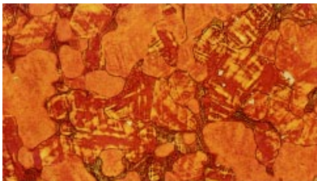
Fig. 16 - Microstructure of as-cast beryllium bronze prepared by the contemporary method (Klemm's I, 100X, bright field).
